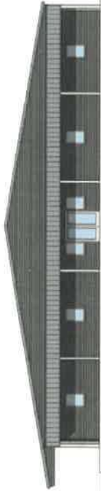
EAST ELEVATION - BUILDING MMM Overall Elevation Width: 90'-0" Distance between Pilasters: 16'-6" Building Height at Eave: 12'-0" Building Height at Peak: 19'-6"
