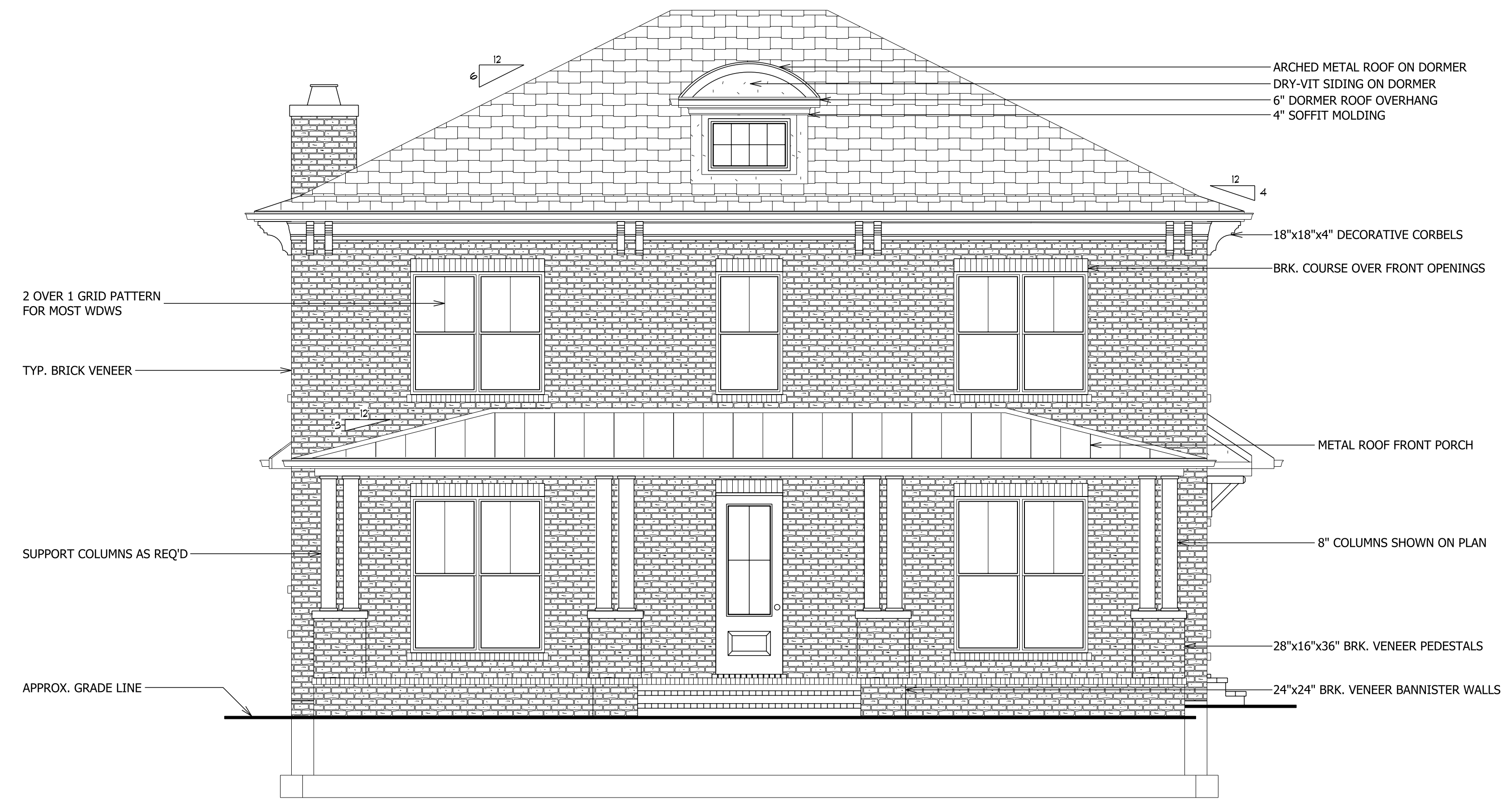
FRONT ELEVATION SCALE: 1/4" = 1'
